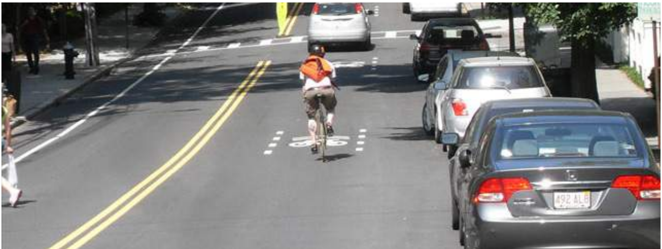
Example of Shared Lane or Sharrow
