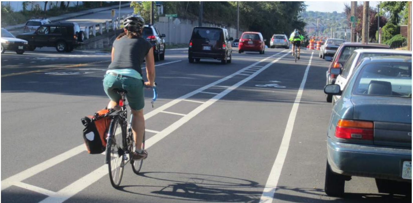
Example of Buffered Bike Lanes
